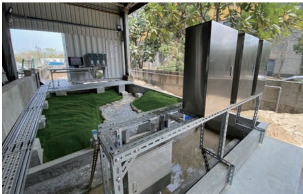
Fig. 1 a & b Dam Control Systems Cybersecurity Testbed
